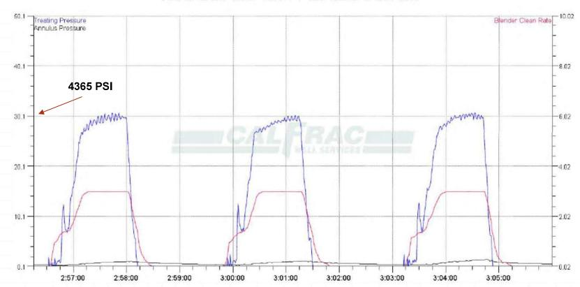
30 bbl/stage of 28% HCL Pumped at 19 bbl/min
